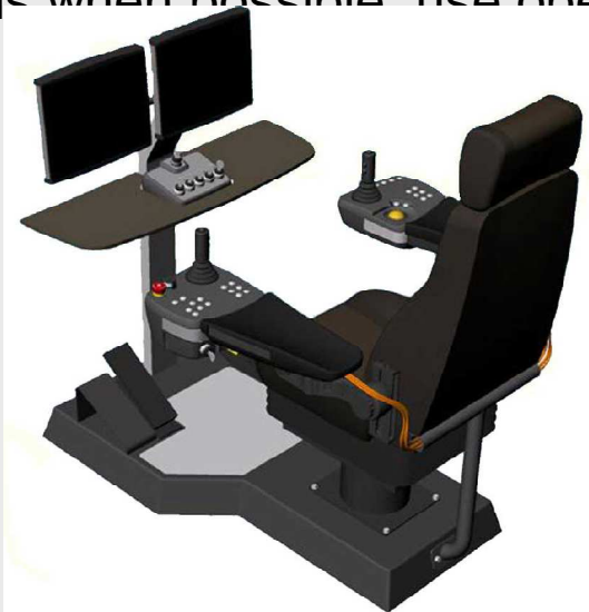
UGM Loading remote operation station
