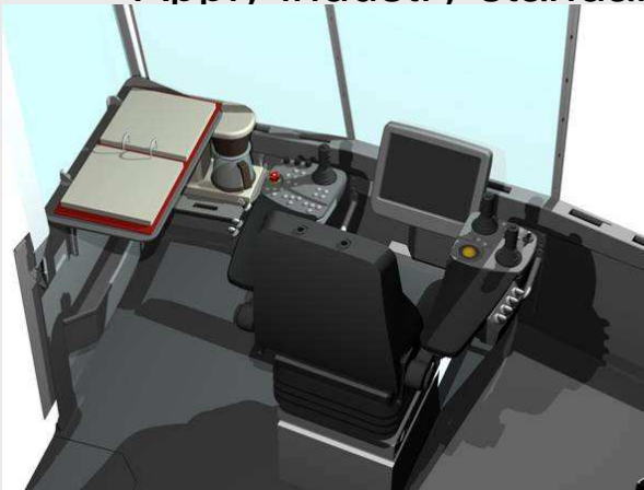
Construction Tunnelling Drill Jumbo
